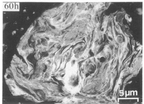
Figure 12 Layered structures observed in the milled powders of the \text{Cr}_2\text{Nb} system after different milling times.
